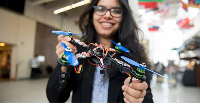
Electrical Engineering student Fizza Ahmad Sheikh and her fourth-year Capstone team developed the First In Risk Evaluation (FIRE) System to help improve the safety of firefighting operations. By piloting a drone equipped with thermal imaging cameras, firefighters are able to measure heat intensity and identify structural dangers through a specialized graphic user interface.
