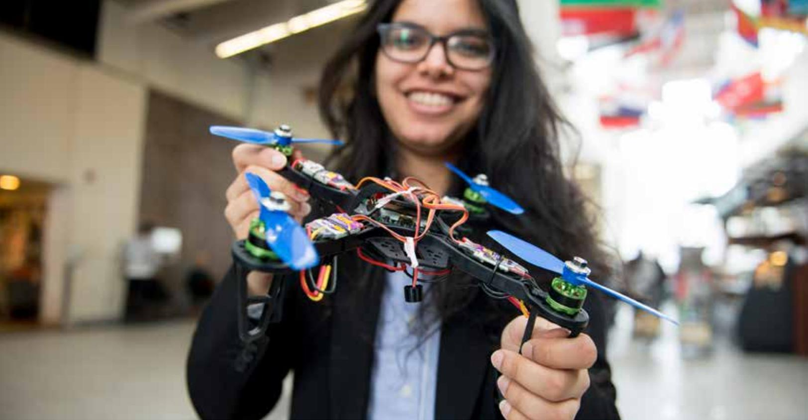
Electrical Engineering student Fizza Ahmad Sheikh and her fourth-year Capstone team developed the First In Risk Evaluation (FIRE) System to help improve the safety of firefighting operations. By piloting a drone equipped with thermal imaging cameras, firefighters are able to measure heat intensity and identify structural dangers through a specialized graphic user interface.
